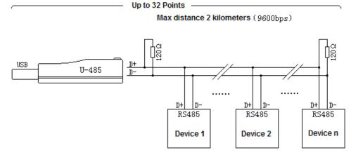
1, Shielded twisted pair with. above 0.5 mm2 cross-sectional area and 120-ohm impedance should be used as the communication lines,
