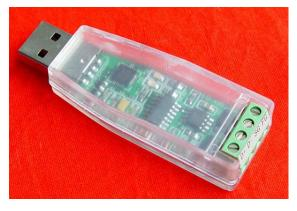
which is different from other similar cheap products in market. There is a built-in anti-static antilightning circuit in the product. This product for micro-design, size is as the same with the flash, antistatic and anti-lightning circuit was built-in, uniquely with sending/receiving indicator lights.
