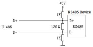
The 120  $\Omega$  resistances in the picture is terminal resistance. They are to prevent the signal reflection in the line. 1 K resistances are the level-pull-up resistor and level-pull-down resistor respectively. Its role is to ensure the line is logic "1" when the line is in leisure so that the data bits in cease - to prevent the reception error.
